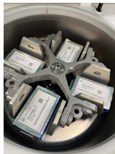
Figure 3. qRePS panels. Each qRePS panel contains the full set of heavy-labelled protein-fragment standards in every well, enabling multiplex, multi-peptide quantification of the targeted proteins. The dried format supports consistent sample handling and facilitates integration into both manual and automated workflows. Stability at ambient temperature also simplifies storage and transport.
