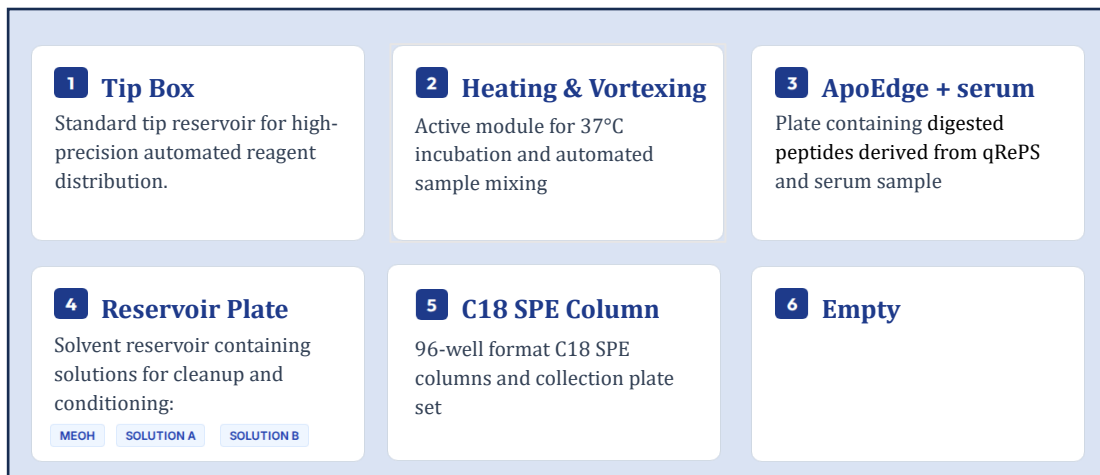
Figure 4: Layout of plates, tips, and heating block on the Hudson SOLO Automated Liquid Handler during the solid-phase extraction procedure.
