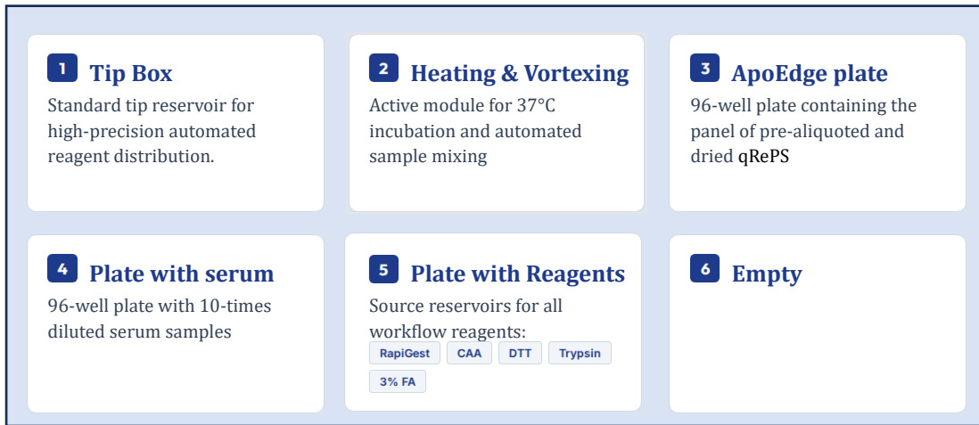
Figure 2: Layout of plates, tips, and heating block on the Hudson SOLO Automated Liquid Handler during the digestion procedure.
